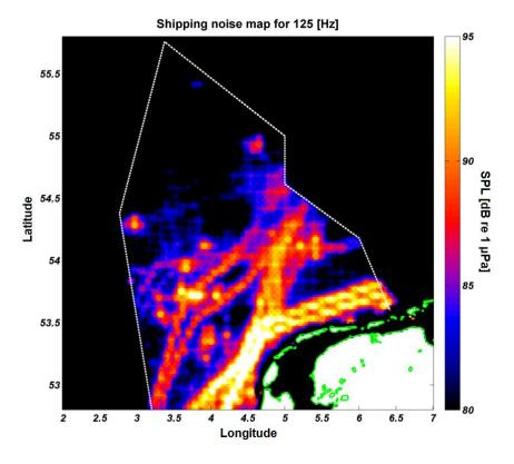
Figure 1: Shipping sound map of unweighted SPL [dB re 1 μPa] in the 1/3-octave band centred at 125 Hz (Annex F). Green border indicates the land boundary and white border the Exclusive Economic Zone (EEZ) of the Netherlands. X and Y axes indicate longitude and latitude, respectively.
